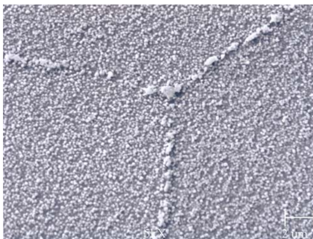
Fig. 4 Typical microstructure for the fully wrought condition at 5000x
